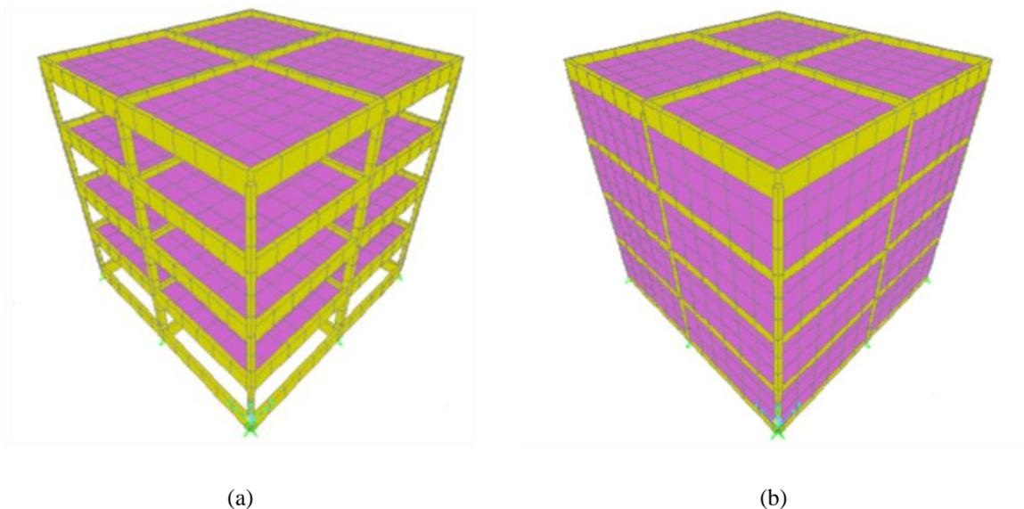
Figure 2. (a) Three-dimensional model of the building without discretized masonry walls (masonry walls incorporated as distributed load) and (b) Model with discretized masonry walls
