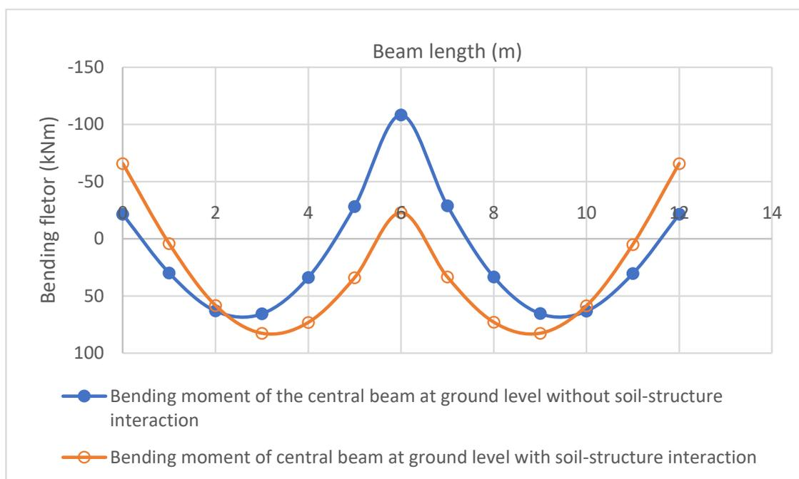
Figure 6. Bending moment diagram of the central beam at ground level, without considering soil-structure interaction and with interaction
