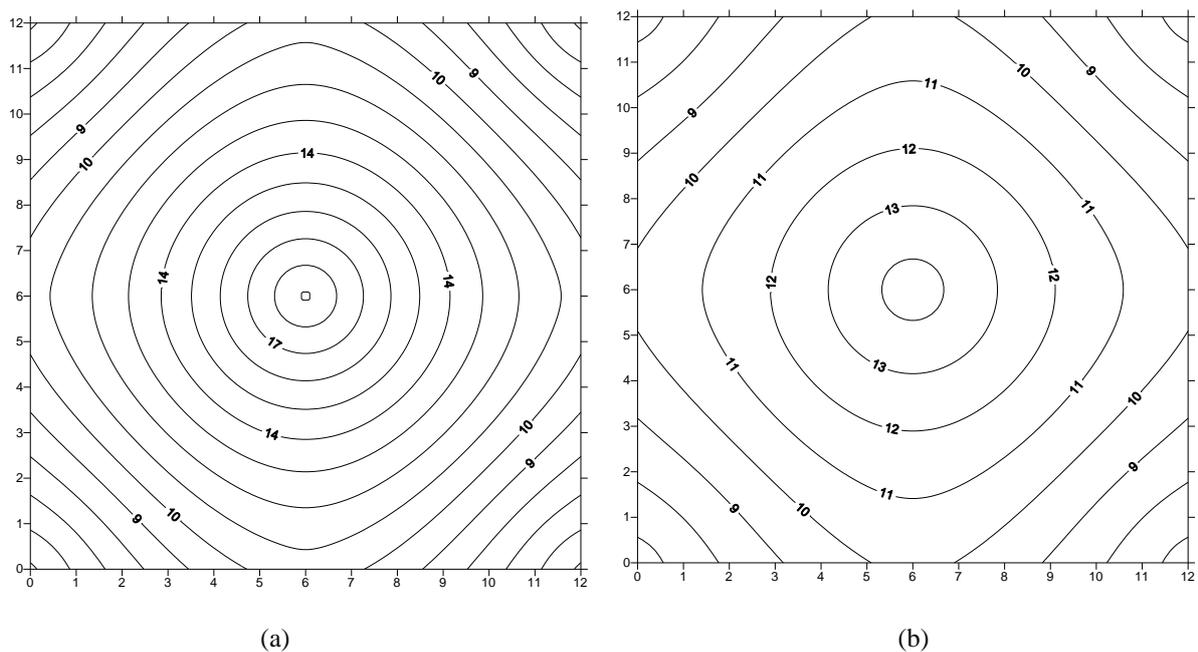
Figure 5. Settlement basin for the model with discretized masonry walls (a) without considering the soil-structure interaction and (b) with the interaction
