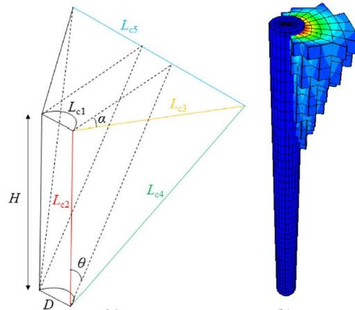
Figure 2: Example of analysis of a failure wedge, showing a theoretic scheme and a 3D finite element post processing for a cylindrical foundation [15].
