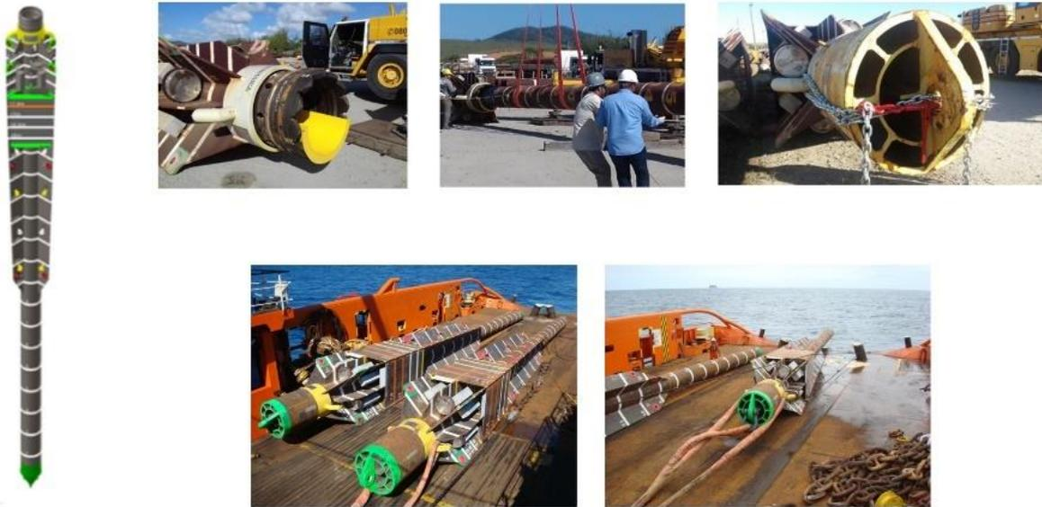
Figure 1. Pictures of a torpedo base being handled and in the deck of an AHTS vessel. (Source: Petrobras)
