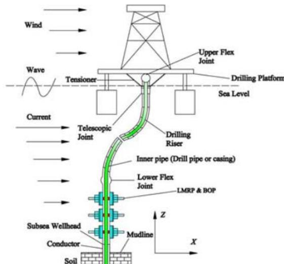
Figure 3: Schematic of a fully coupled drift off analysis in a dynamic positioning drilling rig [17].
