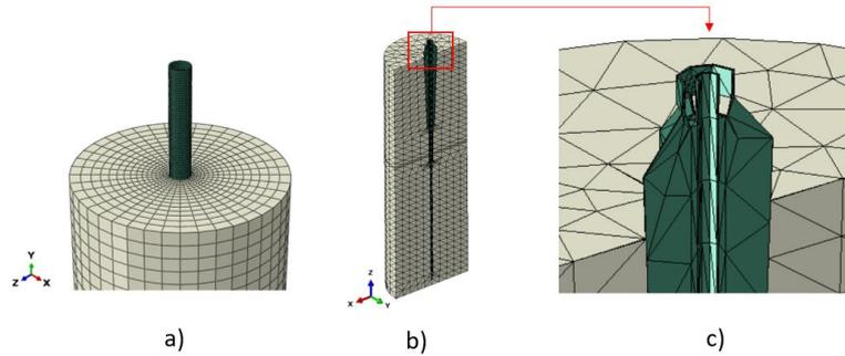
Figure 5: Jetted Conductor Mesh (a) and Torpedo Base Mesh (b) Zoomed View of Torpedo Mesh (c)
