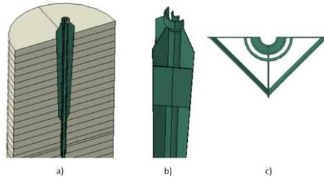
Figure 4: Multilayered Soil in Contact with Torpedo Base (a) Focus on Symmetry (b) Top View (c)
