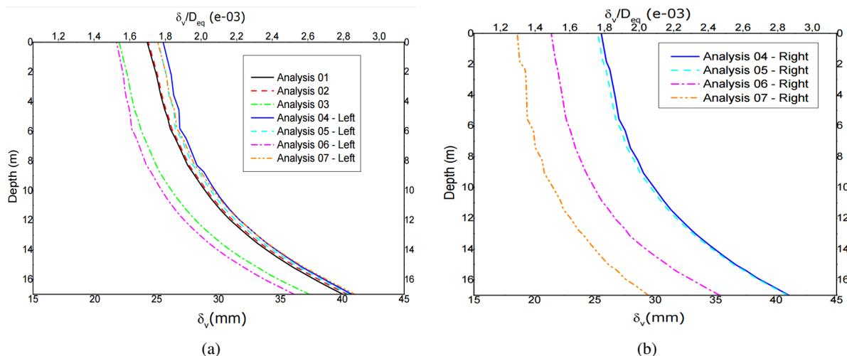
Figure 7. Vertical displacement along tunnel axis (a) left tunnel (b) right tunnel
