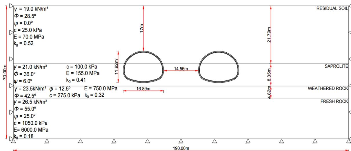
Figure 1. Model geometry
