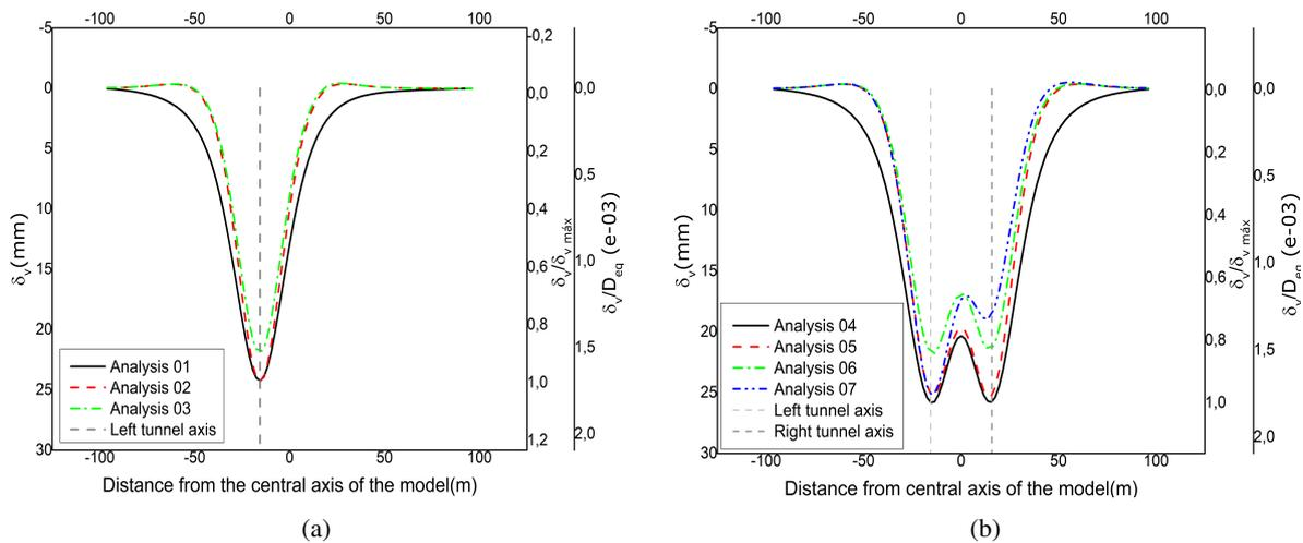
Figure 6. Surface settlement to each analysis (a) single tunnel (b) twin tunnel
