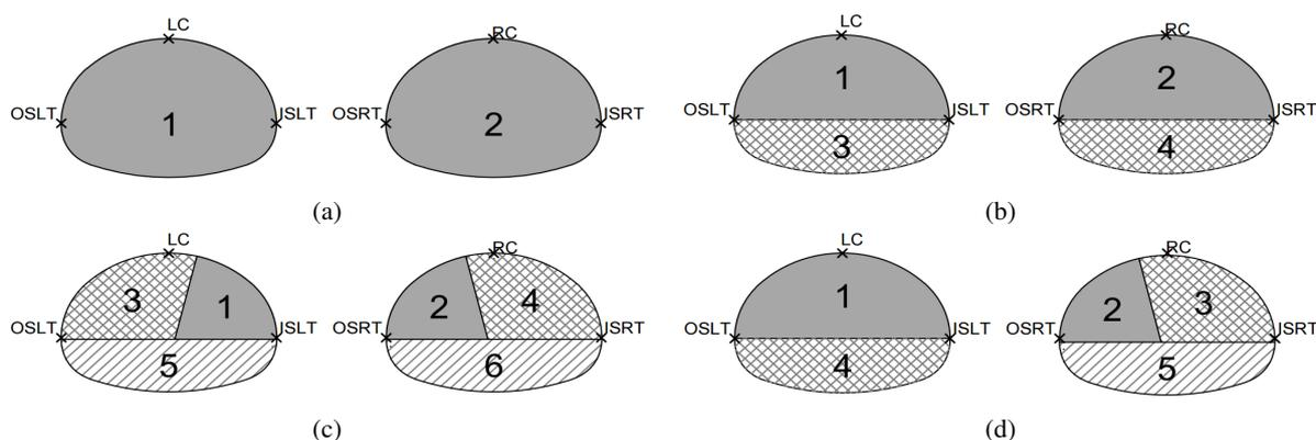
Figure 4. Excavation sequence twin tunnel (a) Analysis 04 - full face excavation, (b) Analysis 05 - crown and invert excavation, (c) Analysis 06 - side drift, half section and invert excavation and (d) Analysis 07 - crown and invert excavation for the left tunnel and side drift, half section and invert excavation for the right tunnel
