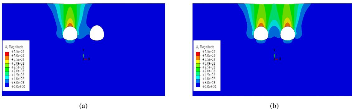
Figure 5. Typical displacement field (a) single tunnel (b) twin tunnel
