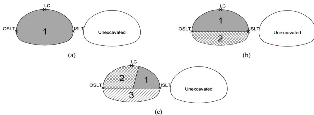
Figure 3. Excavation sequence single tunnel (a) Analysis 01 - full face excavation, (b) Analysis 02 - crown and invert excavation, (c) Analysis 03 - side drift, half section and invert excavation
