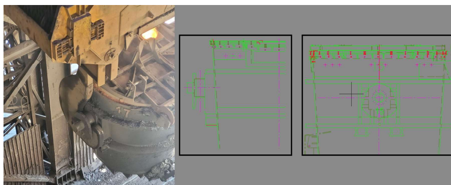
Figure 3. Trunnion guide for hook alignment
