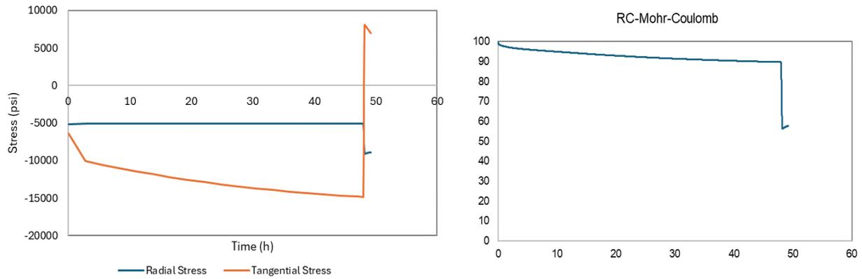
Figure 4. Stresses during curing (first 48h) and blowout event (at the end) at left. Remaining capacity for Mohr-Coulomb criteria on right
