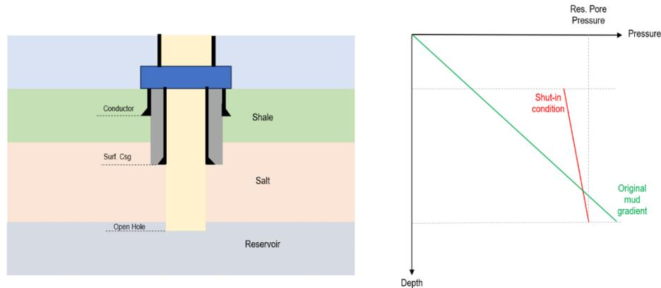
Figure 1. Well condition and load case for containment evaluation (Source: Authors)
