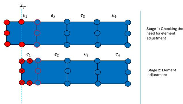
Figure 2. Steps for adjusting the last element
