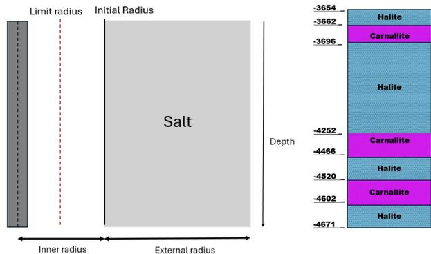
Figure 6. Well geometric properties and lithology (Halite and carnallite)
