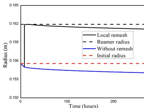
Figure 8. Well displacement field with/without element adjustment (local remesh).
