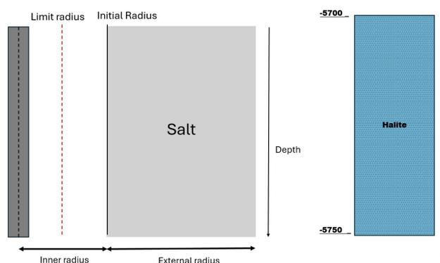
Figure 3. Well geometric properties and lithology (Halite)
