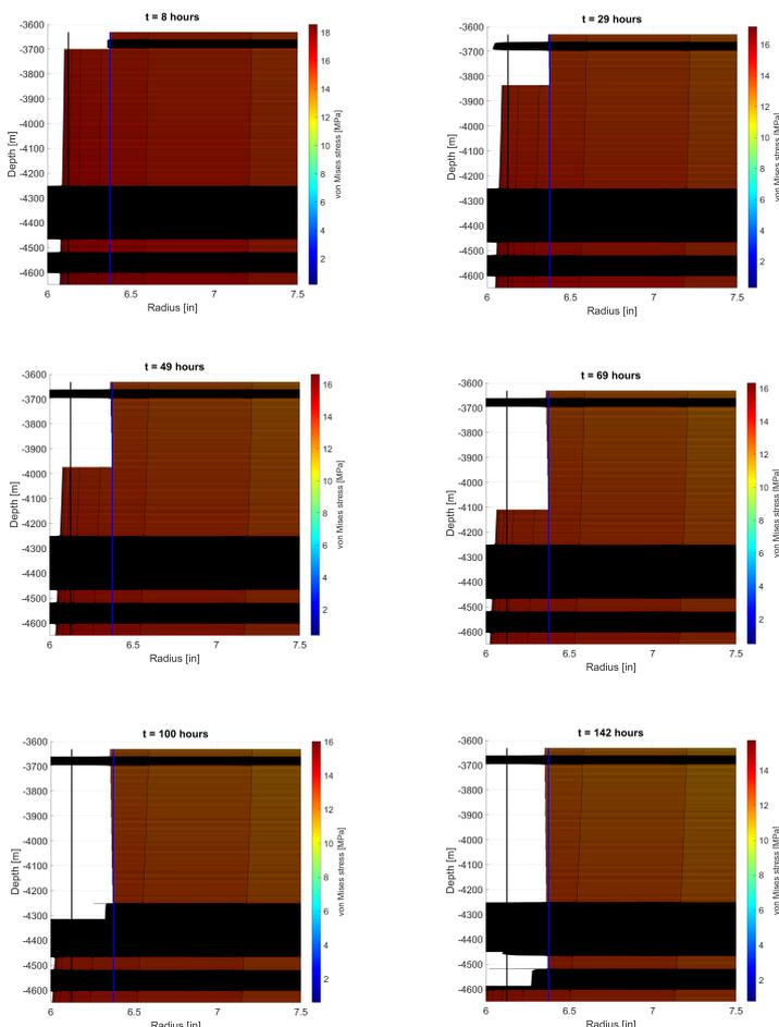
Figure 7. von Mises stress for the methodology considering local remesh
