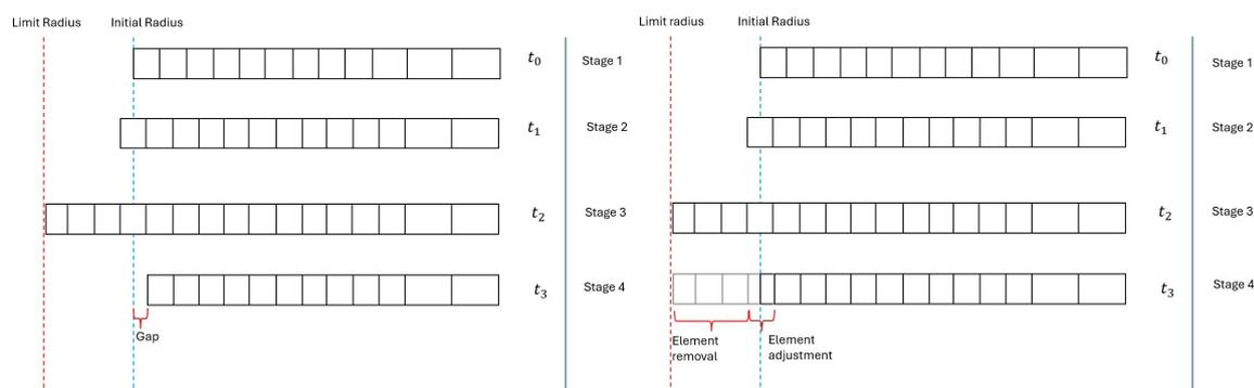
Figure 1. Gap between the initial radius and the first node after reaming (left picture) and the element adjustment (right picture)
