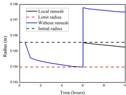
Figure 5. Well displacement field considering the methodology with/without element adjustment (local remesh).
