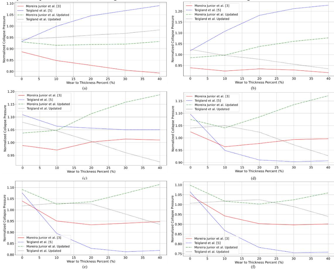
Figure 1. Normalized collapse pressure for (a)  $OD/wt$  equal to 12.0, (b)  $OD/wt$  equal to 16.0, (c)  $OD/wt$  equal to 20.0, (d)  $OD/wt$  equal to 24.0, (e)  $OD/wt$  equal to 28.0, and (f)  $OD/wt$  equal to 32.0
