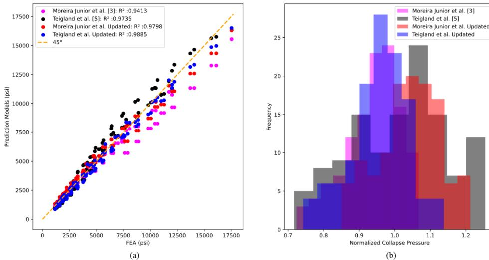
Figure 2. Comparison to FEA results: (a) FEA vs. Prediction Models collapse pressures and (b) Histogram of normalized collapse pressures.
