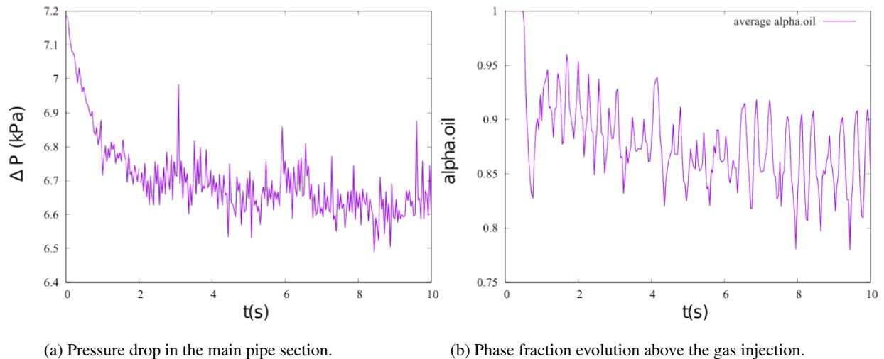
Figure 2. Total pressure drop and phase fraction over time for 53k mesh.
