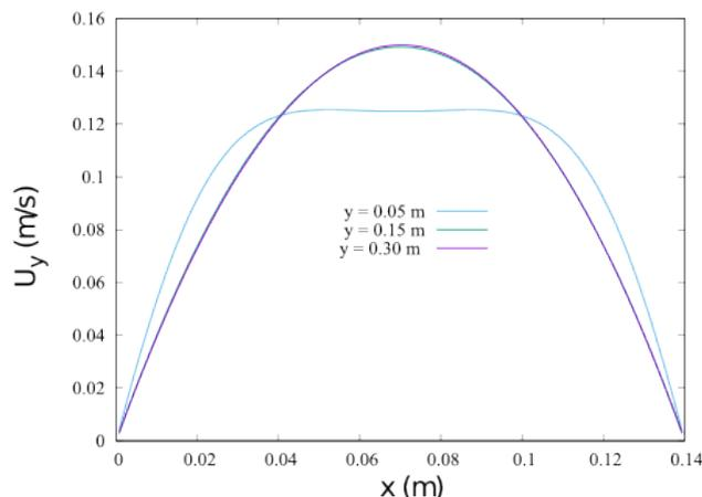
Figure 3. Velocity profile in the entry region (mesh 186K).
