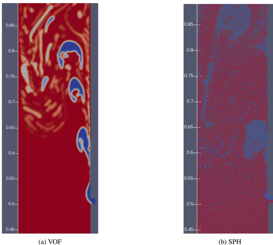
Figure 4. Snapshot of the main flow section at  $t = 5.0$  s, with the VOF method and the SPH method.
