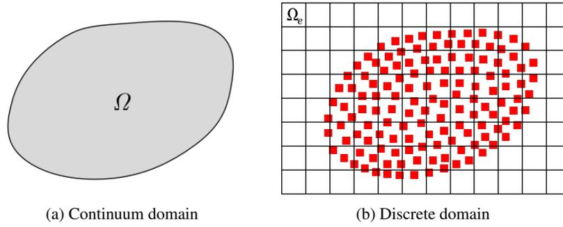
Figure 1. Discretization of the physical domain in GIMP. In this method, the continuum domain (a) is represented by a set of material points (or particles), represented in the color red (b). Alongside the particles, a fixed background grid is created. As the background grid remains still during the simulation, it must cover the entire region that the particles may occupy.
