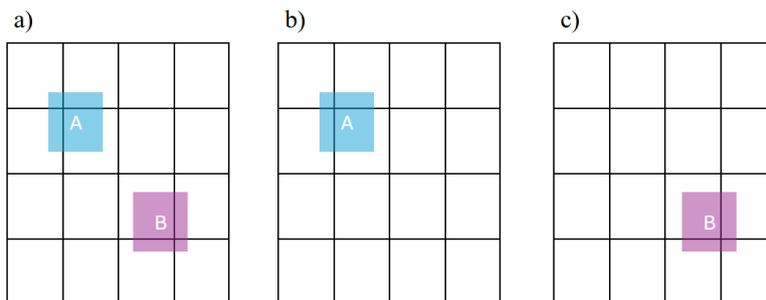
Figure 3. Primary-secondary contact algorithm. a) Primary grid. b) Second A grid. c) Secondary B grid.
