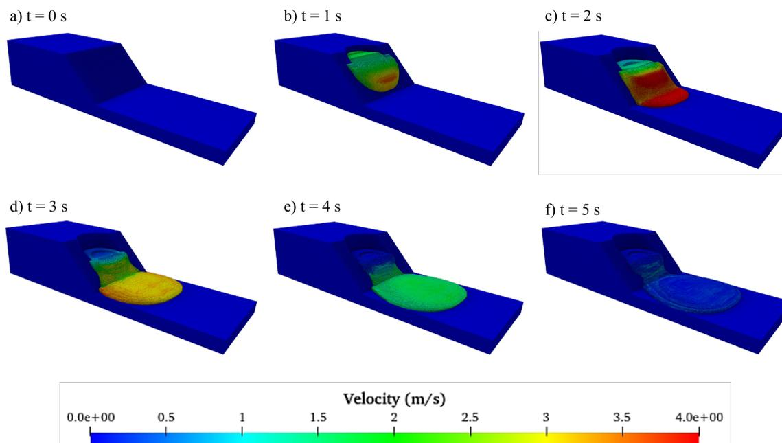
Figure 6. Landslide flow timeline with emphasis on the magnitude of the velocity field
