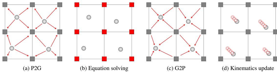
Figure 2. The four basic steps in a typical GIMP time step. a) Particle data is mapped to the background grid (P2G). b) The equations of motion are solved in the background grid. c) Grid results are mapped back to the particles. d) Update of particle kinematics with the mapped results.
