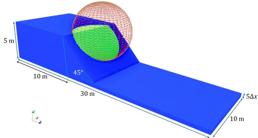
Figure 5. Schematics of the submarine landslide model with display of the critical slip surface geometry and model dimensions
