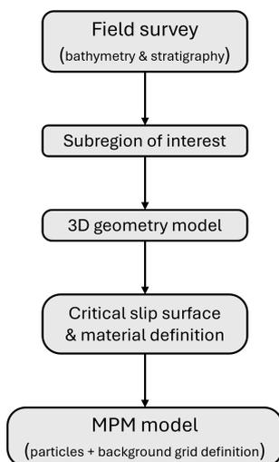
Figure 4. Submarine landslide modelling workflow
