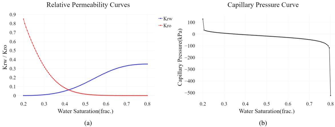
Figure 3. Relative permeability (a) and capillary pressure (b) curves used in the simulations.
