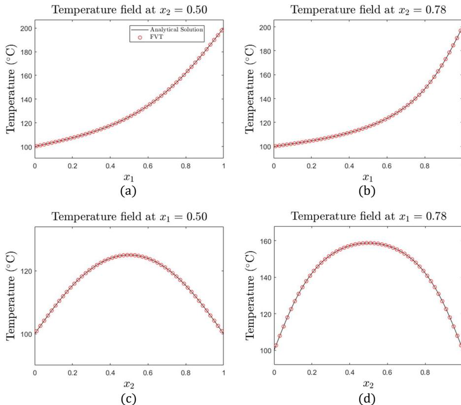
Figure 4: Comparison of the surface-averaged temperatures on the faces of the subvolumes with the results obtained from the analytical solution: (a)  $x_2 = 0.50$ , (b)  $x_2 = 0.78$ , (c)  $x_1 = 0.50$  and (d)  $x_1 = 0.78$ .
