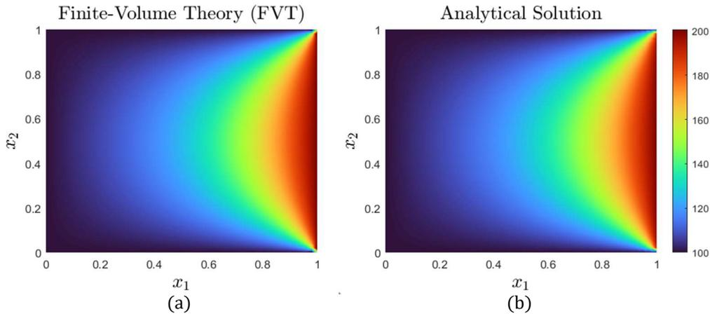
Figure 3: Temperature field: (a) FVT with 50x50 mesh of subvolumes and (b) analytical solution.
