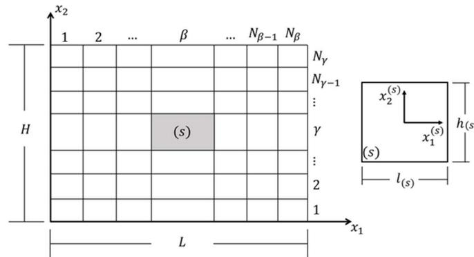
Figure 1: Discretized analysis domain in rectangular subvolumes and local coordinate system of a generic subvolume.
