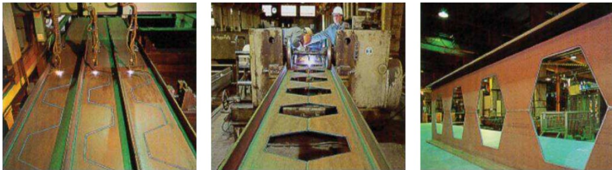
Figure 1. Manufacturing process of castellated beams [3].
