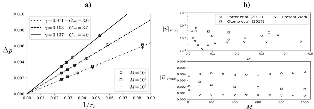
Figure 3. Superficial tension and spurious currents: a) Laplace equation verification for different values of  $M$  and  $G_{\sigma\bar{\sigma}}$ ; b) Comparison of the max value of spurious currents in function of  $\nu_1$  and  $M$ .
