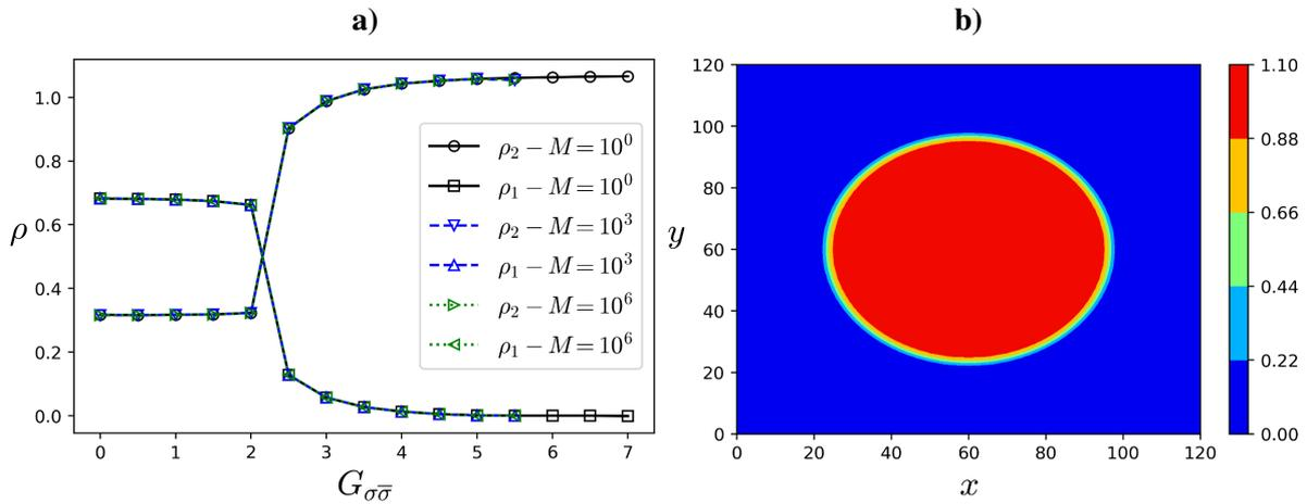
Figure 2. Immiscibility test: **a**) variation of the density  $\rho_1$  and  $\rho_2$ , in the center of the volume for different values of  $G_{\sigma\bar{\sigma}}$  ( $M = 10^0$ ;  $M = 10^3$ ;  $M = 10^6$ ); **b**) density field in the immiscible range.
