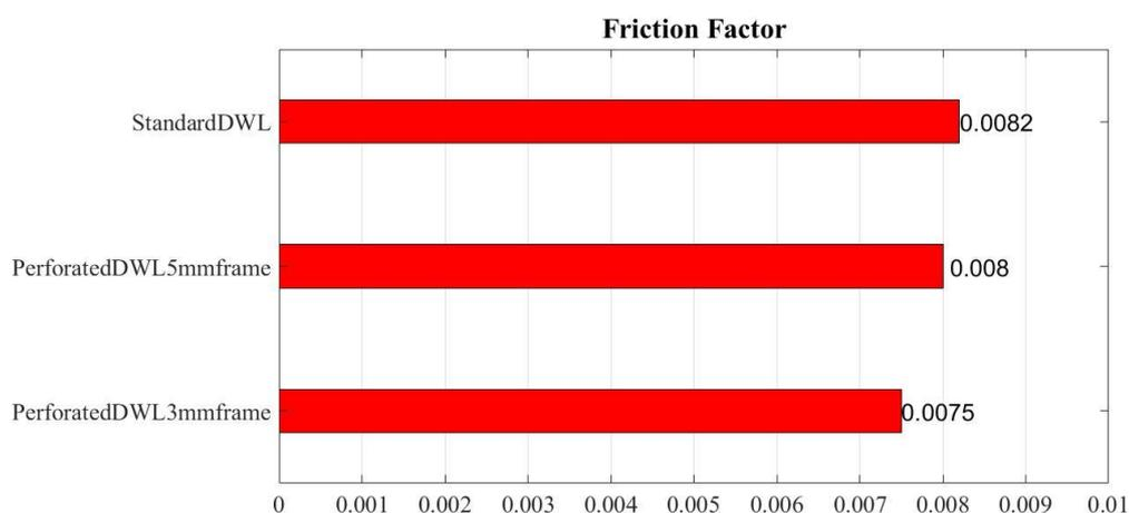
Figure 9. Friction factor for the three DWL pair geometries.
