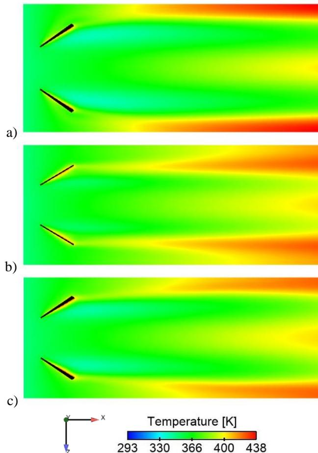
Figure 5. Plate temperature a) Standard DWL b) 3mm frame c) 5mm frame
