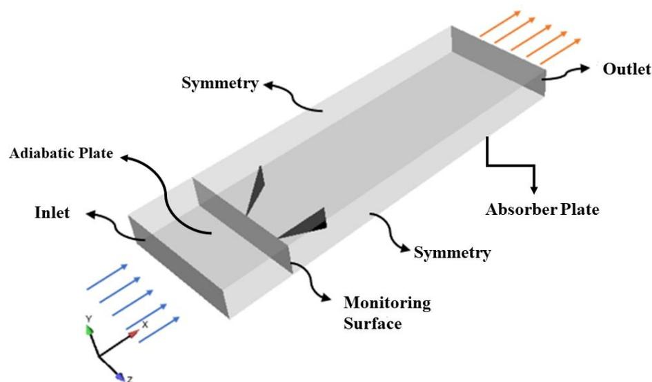
Figure 3. Computational domain; inlet and outlet.
