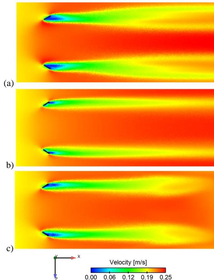
Figure 7. Velocity Plate-to-plate 15mm height a) Standard DWL b) 3mm frame c) 5mm frame
