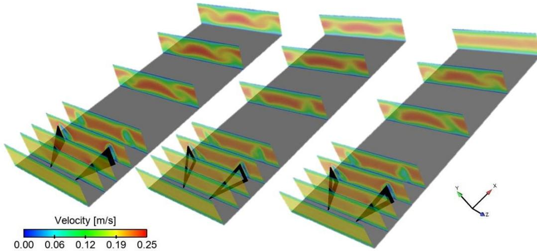
Figure 6. Cross section planes showing the velocity magnitude along the main flow direction for different DWL geometries.
