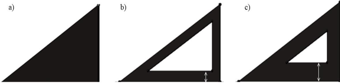
Figure 4. Geometric Modifications: a) Standard DWL; b) Perforated DWL 3mm frame and c) Perforated DWL 5mm frame.
