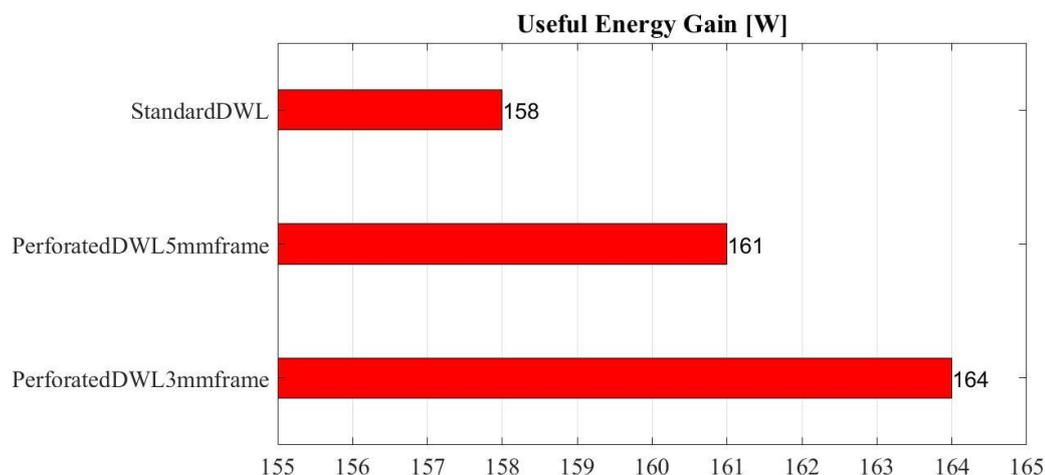
Figure 8. Useful heat gain for the three DWL pair geometries.
