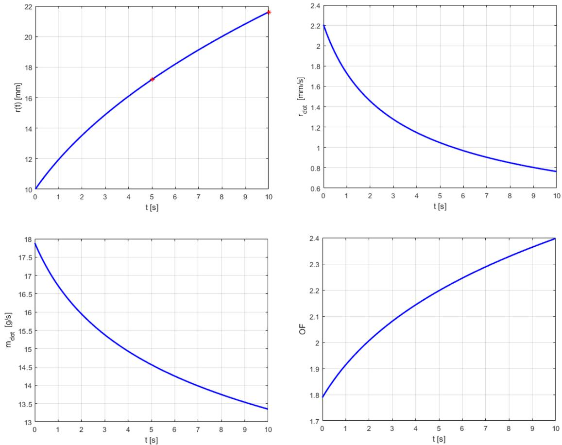
Figure 2. [A] radius, [B] regression rate, [C] fuel mass ow rate, and [D] O/F ratio varying along the burning time.
