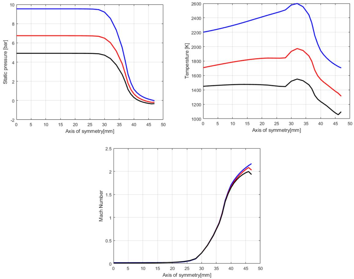
Figure 9. Area-weighted average of the properties pressure, temperature and Mach number along the nozzle.
