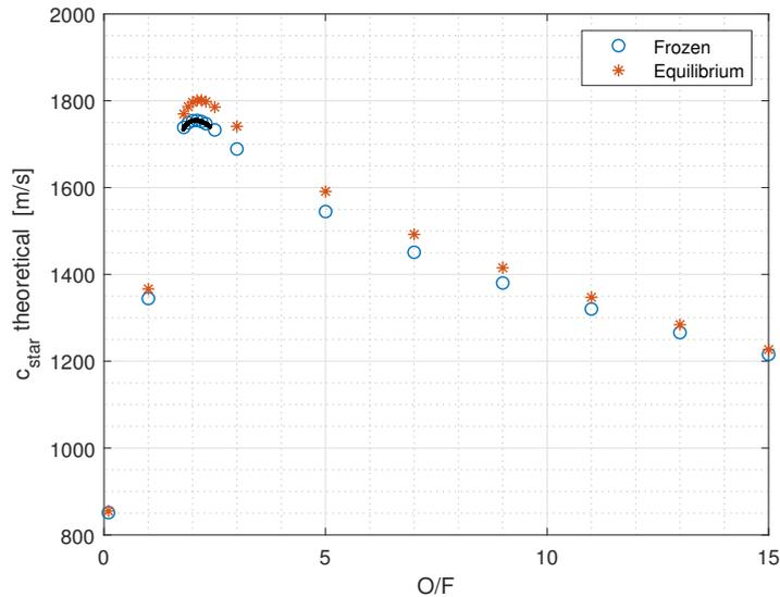
Figure 1. Characteristic velocity varying with O/F ratio at frozen and equilibrium conditions, for a Paraffin/GOX combustion.
