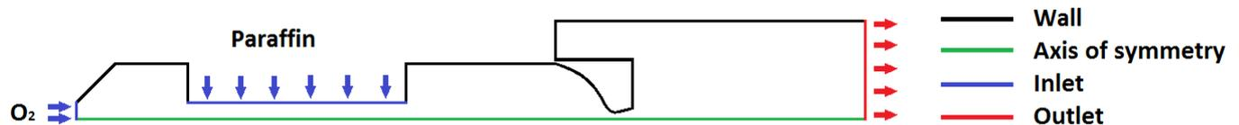
Figure 3. Boundary faces of the combustion chamber and nozzle.
