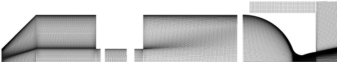
Figure 4. Distribution of the elements in the mesh over all the control volume and near the wall.
