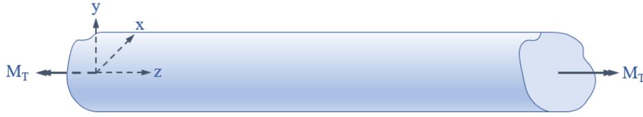
Figure 1. Coordinate system and twisting moment.
