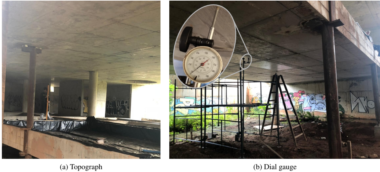
Figure 2. Vertical displacement readings in the first floor test.
