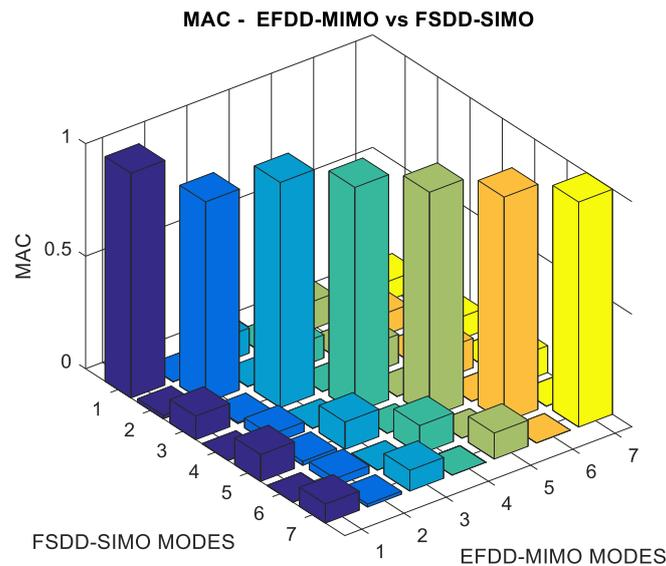
Figure 2. Mode shapes comparison for FSDD-SIMO and EFDD-MIMO
