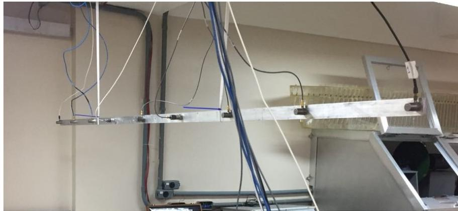
Figure 1. Rectangular aluminum beam and accelerometer positioning in the experiment (accelerometer no. 1 and DOF 1 is in the right side)
