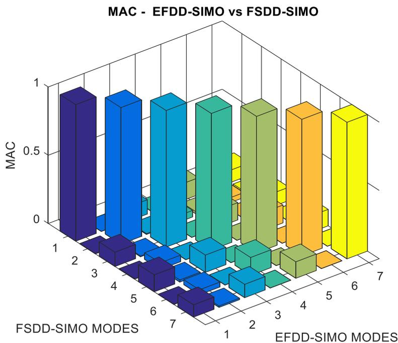
Figure 3. Mode shapes comparison for FSDD-SIMO and EFDD-SIMO
