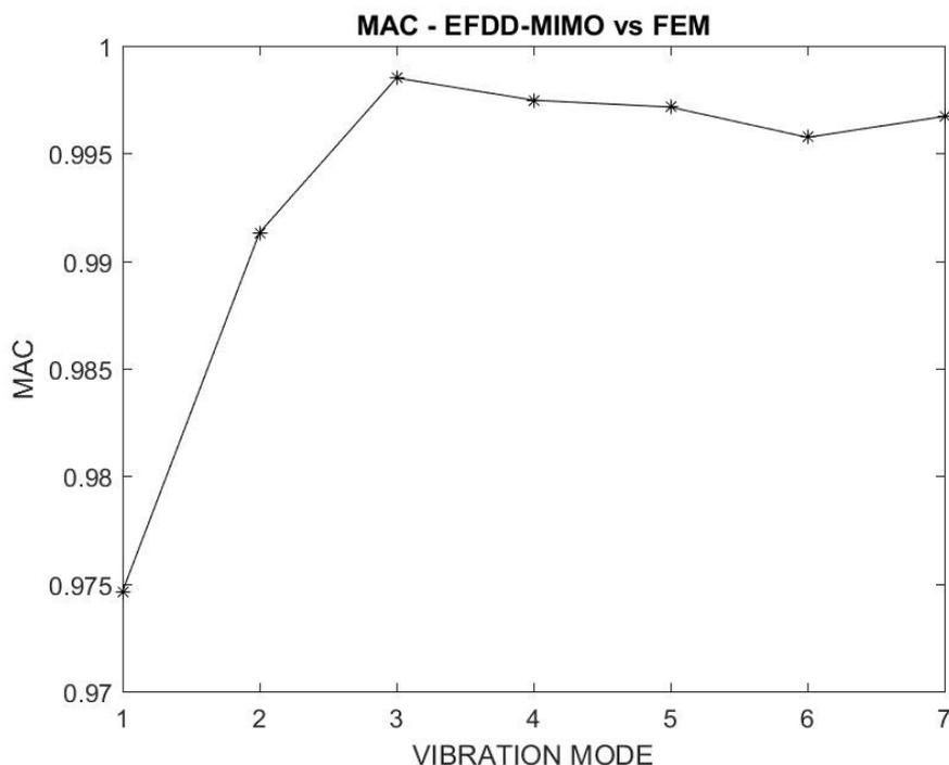
Figure 4. Mode shapes comparison for EFDD-MIMO and FE model
