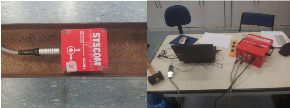
Figure 4 – three accelerometers and SYSCOM acquisition system.
