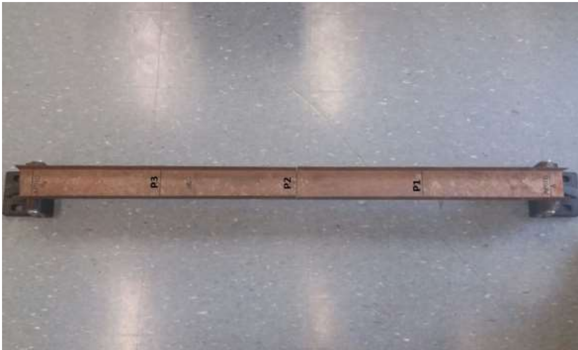
Figure 5 – accelerometers measurement points.
