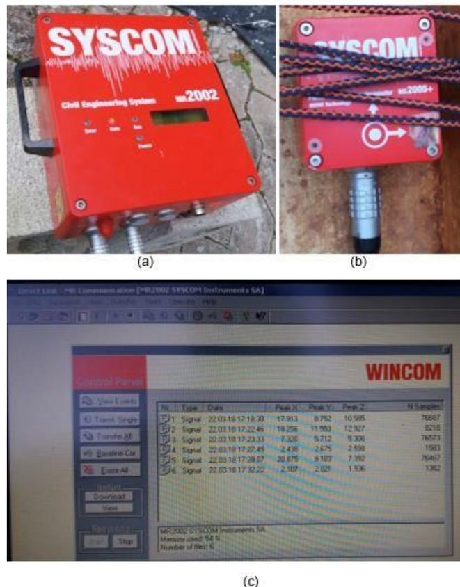
Figura 3. Equipamentos: (a) SYSCOM MR2002; (b) SYSCOM MR2005+; (c) interface do MR communication
