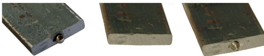
Figure 5. Types of bar termination: embedded sphere, simply filed, embedded pin.
