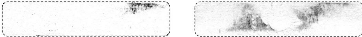
Figure 17: Contact patterns of the simply cut and filed end under two load conditions: 500N and 4kN.
