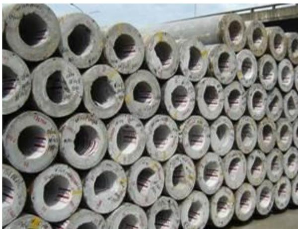
Figure 1. Centrifuged concrete piles (SCAC. Available at: < <http://scac.com.br/>> Access in May 17, 2017.)
