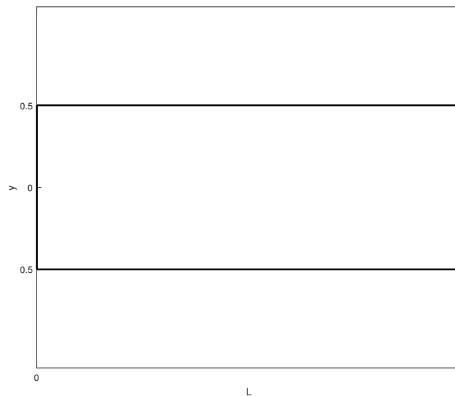
Figure 13. Optimized shape of a hinged-hinged beam that maximizes \omega_1 , \omega_2 and \omega_3 .
