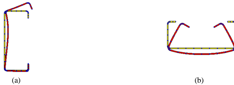
Figure 2. Cross section under distortional buckling: (a) bending about the major axis; (b) bending about the minor axis. Source: CUFSM 5.01 [22].
