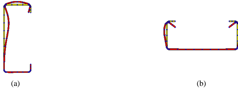
Figure 1. Cross section under local buckling: (a) bending about the major axis; (b) bending about the minor axis. Source: CUFSM 5.01 [22].
