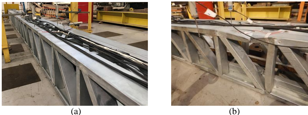
Figure 17: Column T12x0.8, nominal length 12200mm: (a) Local buckling deformation along the chords during the test, (b) collapse mechanism at mid length.
