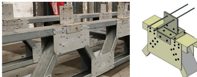
Figure 1. Details of TWP shear connector: (a) during fabrication stage of the full-scale prototype and (b) 3D computational modelling
