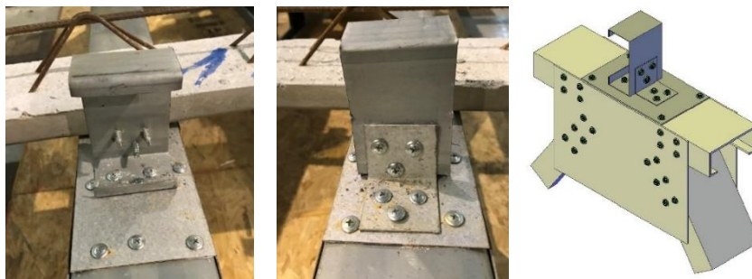
Figure 3. Details of TWC shear connector: (a) front view, (b) back view and (b) 3D computational modelling
