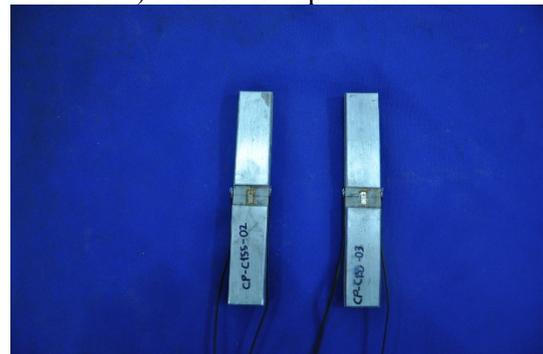
d) Compressive test specimens
