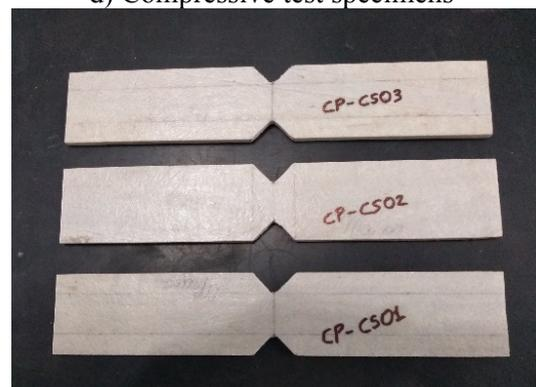
f) Shear test specimens
