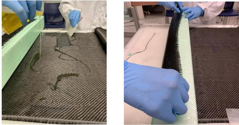
Figure 4. Beam lamination process with resin impregnation in carbon fiber fabric
