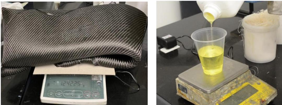
Figure 3. Precision balance used to estimate fiber and resin mass used in beam production
