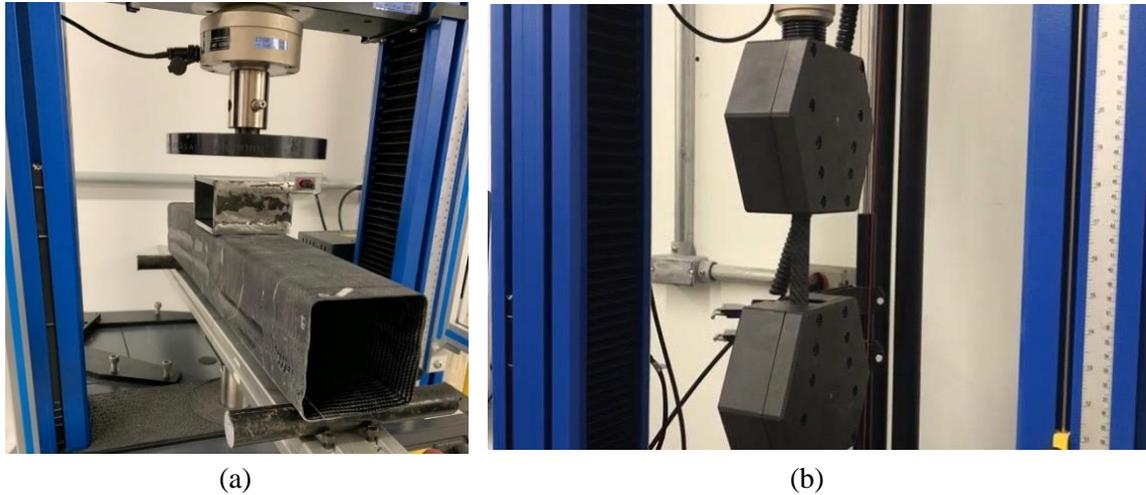
Figure 8. Representation of destructive tests, being (a) flexion and (b) traction
