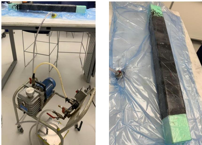
Figure 5. Vacuum pump and vacuum mold / fiber assembly
