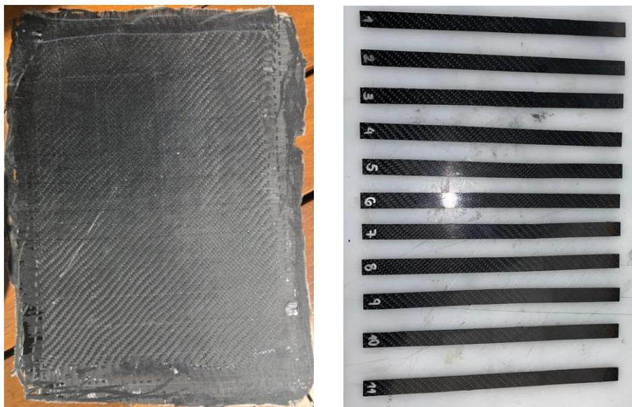
Figure 7. Tensile test plate and specimens
