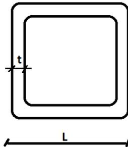
Figure 1. Scheme of beam cross section, with  $L = 100$  mm and  $t$  varying with the number of beam layers
