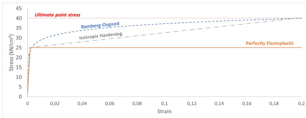
Figure 2. Stress-strain curve of the adopted material according to different plasticity chord
