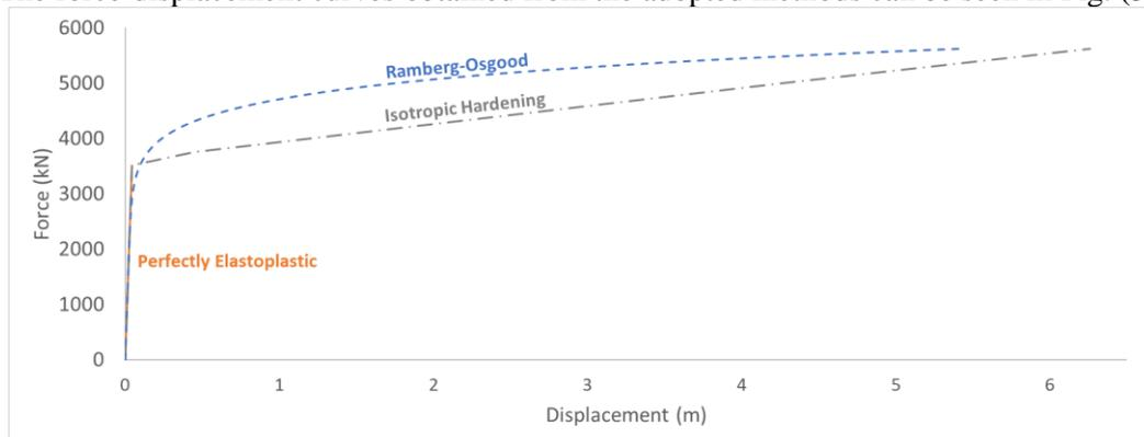
Figure 3. Force-displacement curve for loading applied to the central node of the bottom chord
