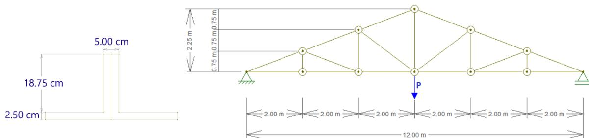
Figure 1. Structural scheme of the analyzed truss with loading applied to the central node
