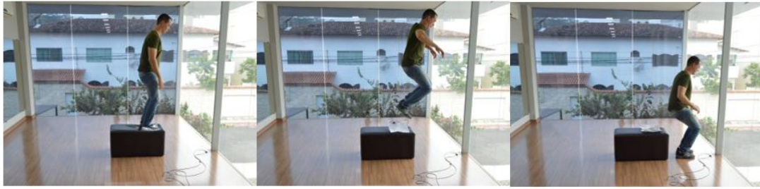
Figure 5. Excitation to induce the first vibration mode of the floor system.
