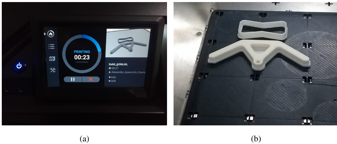
Figure 9. 3D printing process: (a) Stratasys F170 interface, (b) Final printed piece.
