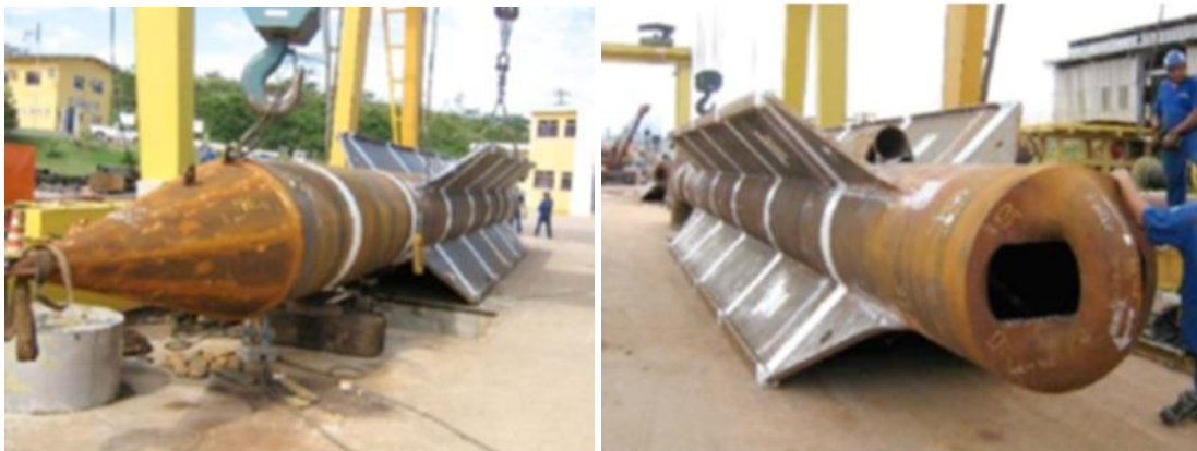
Figure 1. Typical torpedo anchor with four flukes: conical tip (left) and top view with detail of the padeye (right) (Sousa et al. [1]).
