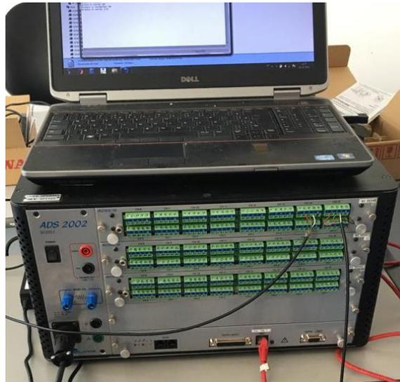
Figure 14. Analog to digital converter (A/D) [personal collection]
