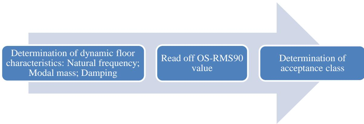
Figure 7. Design process flowchart [personal collection]
