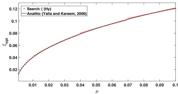
Figure 5. Optimum values of mass ratio  $\mu$  and damping ratio  $\xi$  to minimize response map subject to white noise excitation ( $\alpha = 0.8$ )[3].
