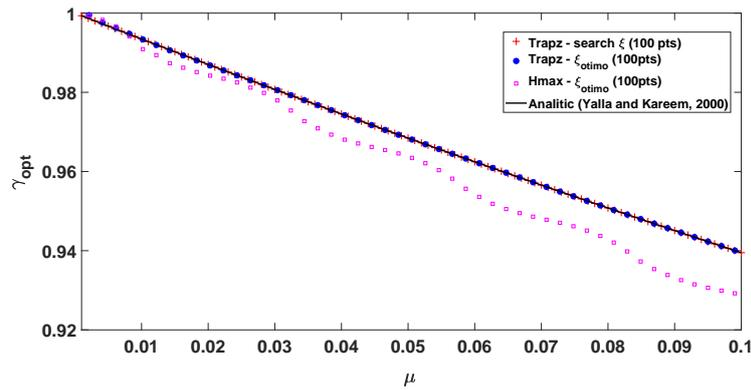
Figure 4. Optimum values of mass ratio  $\mu$  and frequency ratio  $\gamma$  to minimize response map subject to white noise excitation ( $\alpha = 0.8$ )[3].
