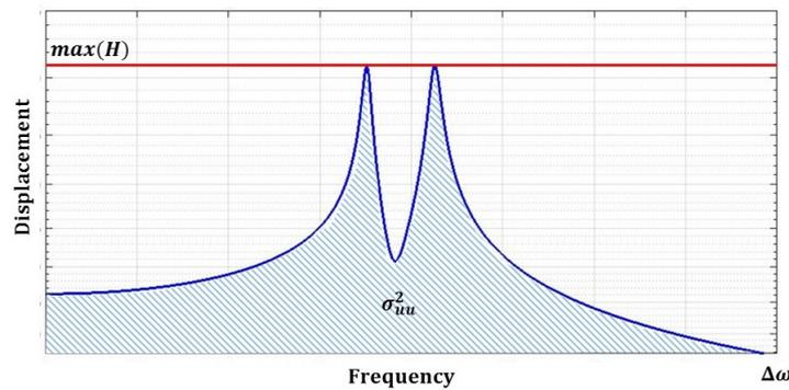
Figure 2. Displacement function of response frequency  $H_u(\Omega)$  as function of frequency  $\Omega$  for coupled mechanical system (main system + TLCD).
