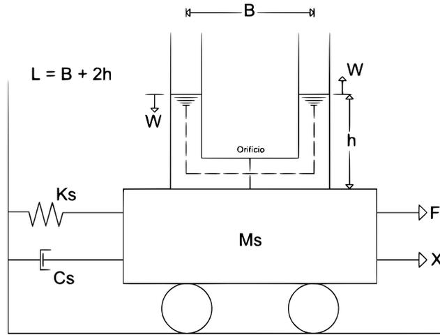
Figure 1. Schematic representation of coupled system main structure and TLCD.
