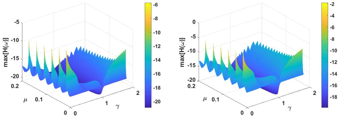
Figure 3. Respose map for white noise with  $\alpha = 0.8$  and  $\xi_s = 0$ . (a) Method 1: Trapezoidal rule (trapz) and (b) Method 2: Hmax
