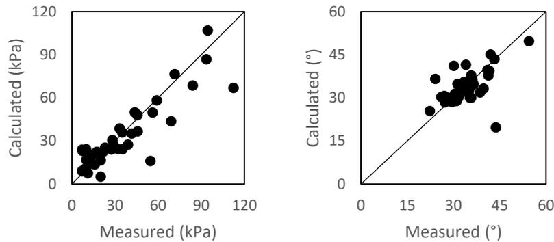
Figure 4. Adjustment of outputs to targets: (a) cohesion prediction; (b) friction angle prediction
