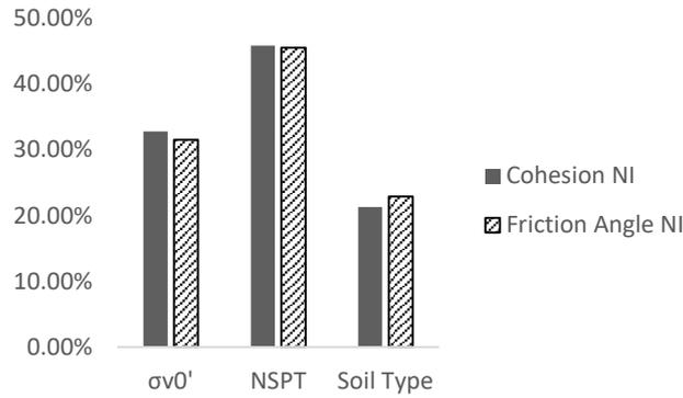
Figure 5. Input node interrogator results for the best model during training for: (a) cohesion prediction; (b) friction angle prediction
