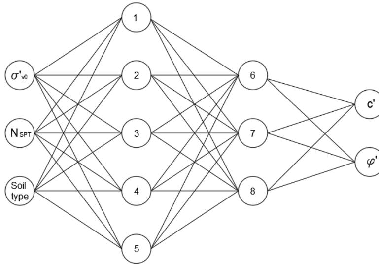
Figure 3. Network architecture of model A:3-5-3-2
