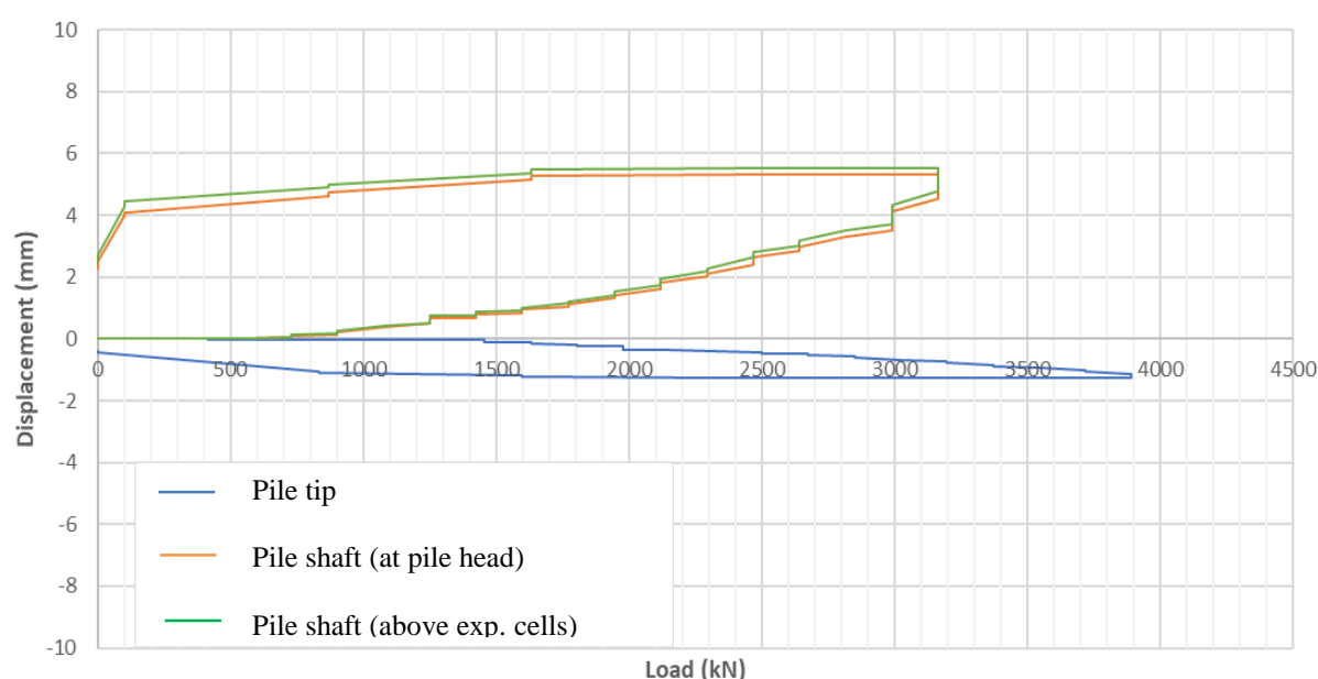
Figure 8. Load x displacement curve (measurement at pile head and above expansive cells)
