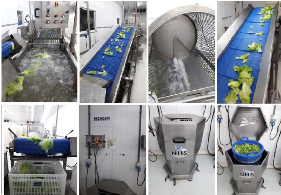
Figure 3. Third and fourth steps: second stream for sanitation, tunnel, leaves conveyor belt and drying process. Source: the author.
