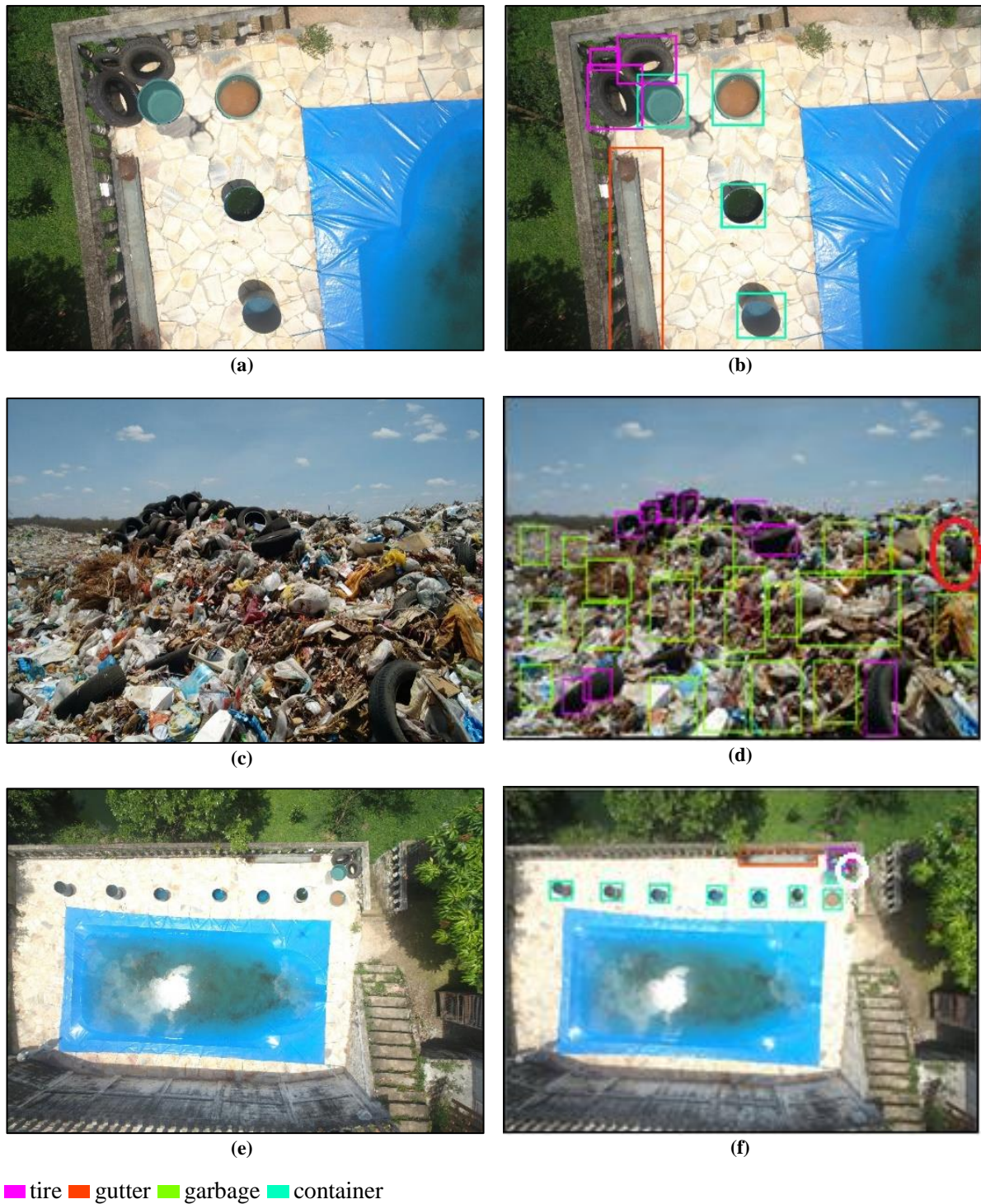
Figure 4. Some results obtained in the task of scenarios detection using CNN_Scenarios
