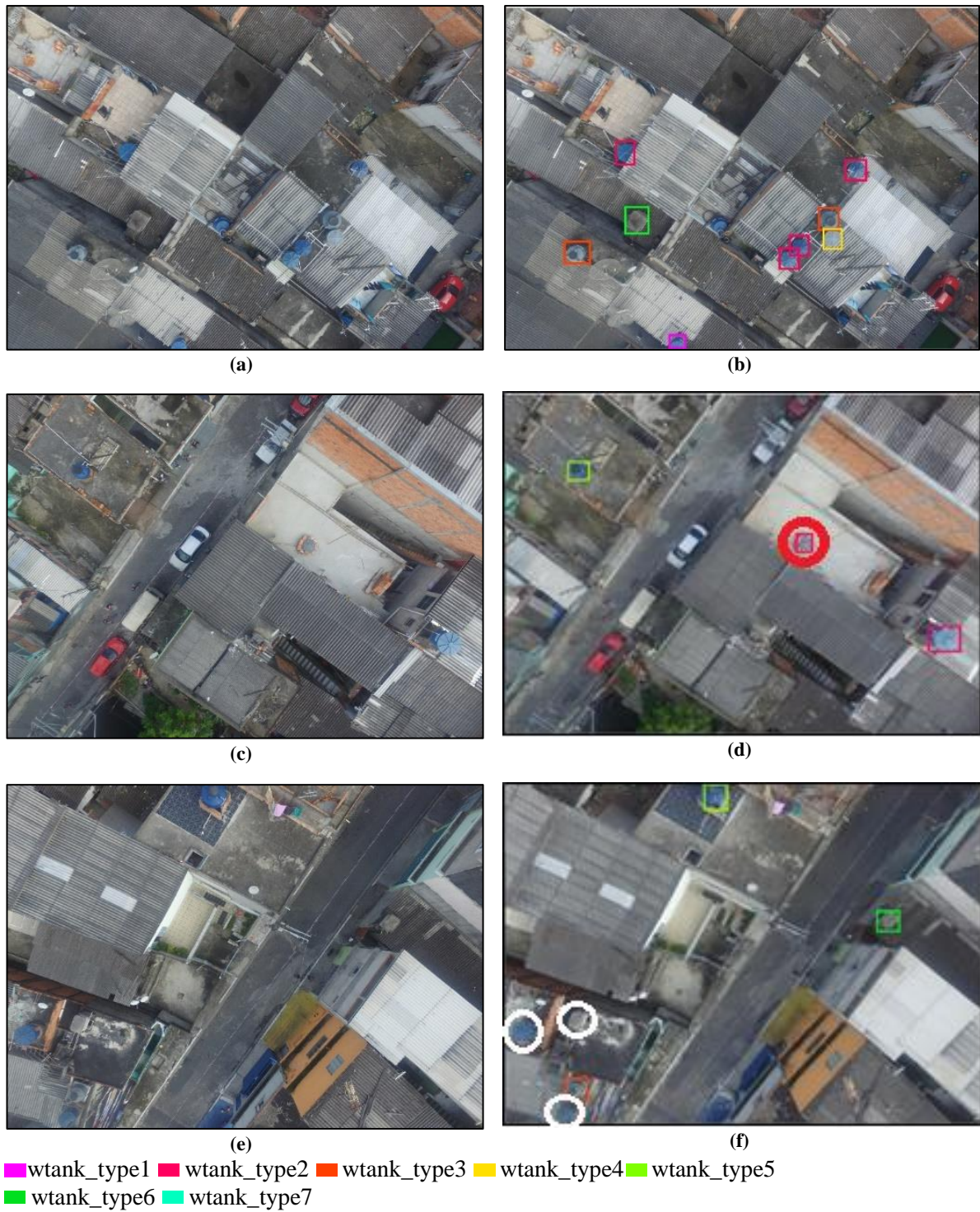
Figure 3. Some results obtained in the task of water tanks detection using CNN_WaterTanks
