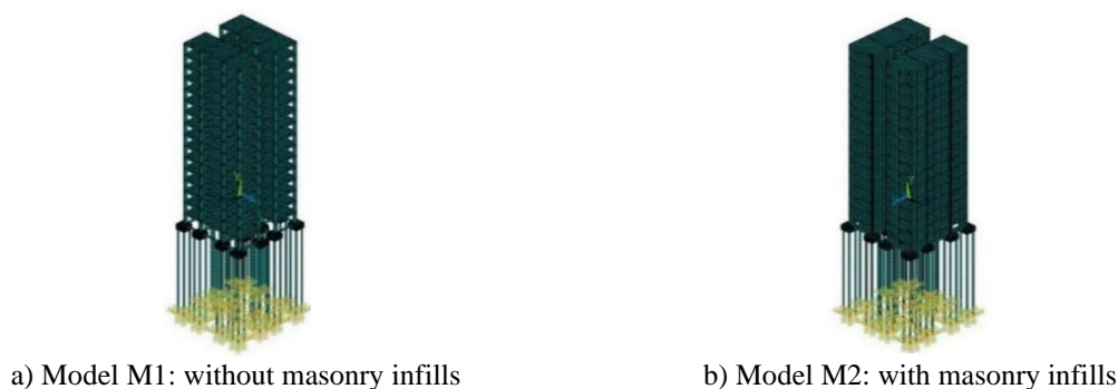
Figure 4. Finite element model of the investigated reinforced concrete building: M1 e M2
