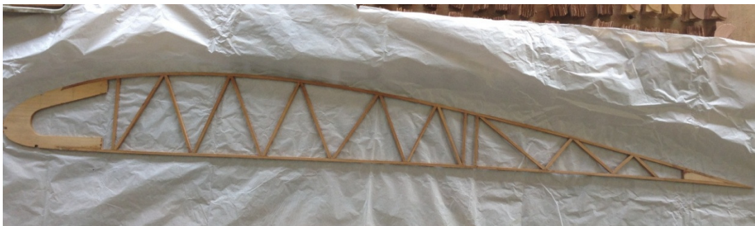
Figure 2. Main airfoil used in Paulistinha
