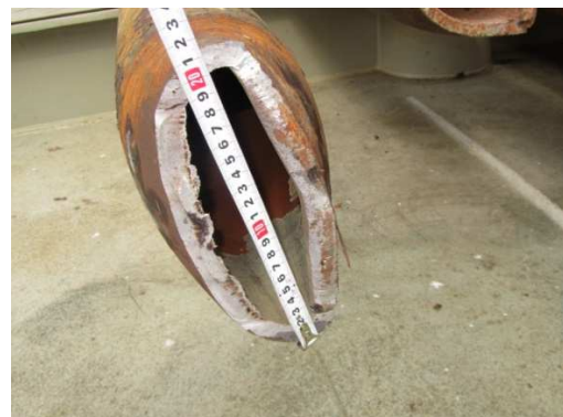
Figure 5 - Drill pipe cut in BOP. Source: Petrobras.
