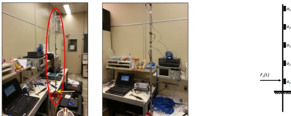
(a) Rectangular beam in cantilever boundary condition and instrumented with 05 accelerometers. (b) Rectangular beam configuration ( F_i : force, a_i : accelerometer).
