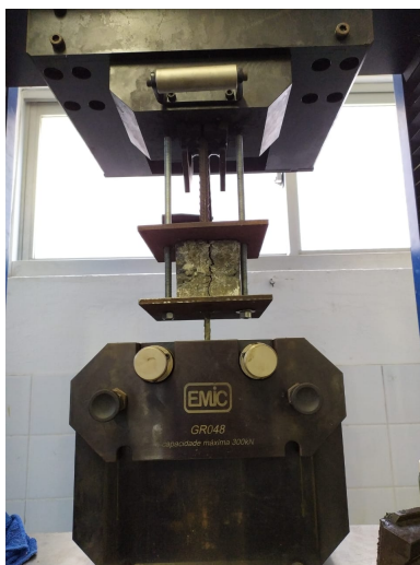
Figure 1. Pullout test experimental equipment
