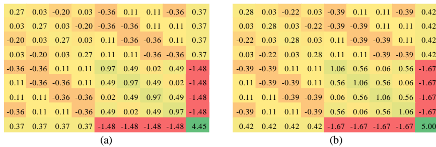
Figure 8. Stability stiffness matrix for quadratic S4 obtained via (a) FEM and (b) approximation.
