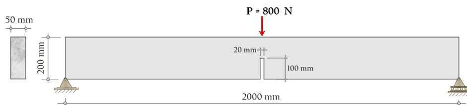
Figure 2. Three-point bending test.
