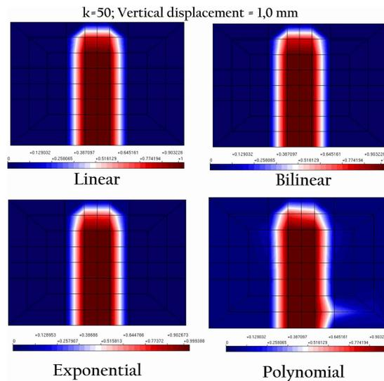
Figure 7. Evolution of damage to the four damage functions: vertical displacement of 1,0 mm.
