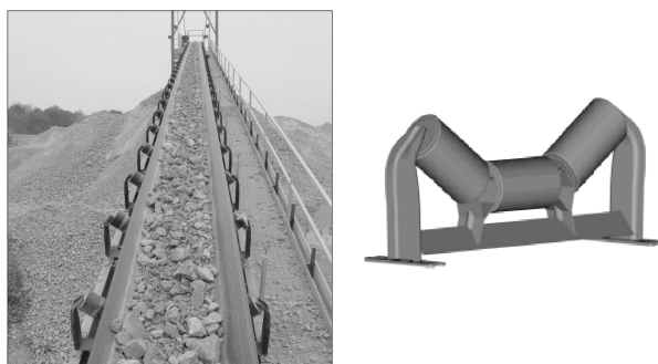
Figure 1. Example of a conveyor belt (left) and a conveyor belt idler with three rollers (right) [1]
