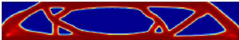
Figure 2. Final topology for the simple supported beam under free vibration (mesh with 240 \times 40 elements and r_{min} = 4 elements)
