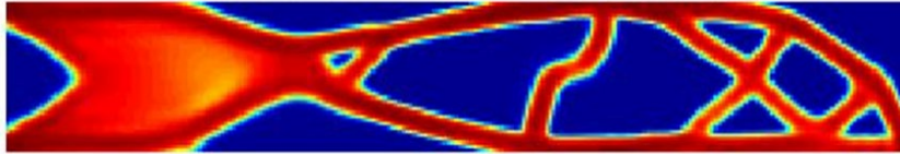
Figure 4. Final topology for the cantilever –supported beam under free vibration (mesh with 240x40 elements and r_{min} = 4 elements).
