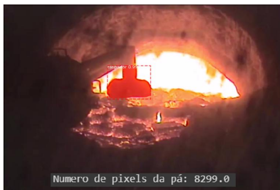
Figure 11. Shovel before replacement
