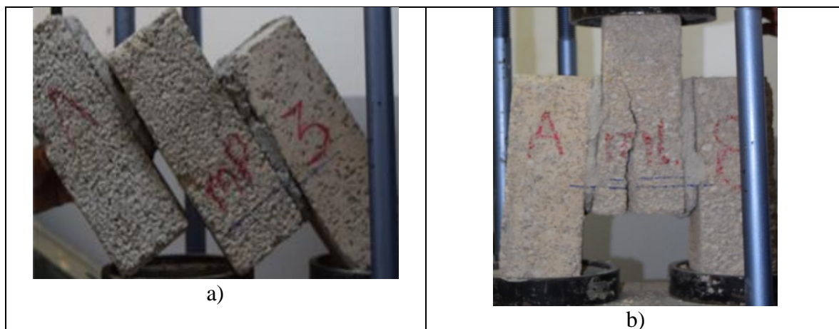
Figure 1. Failure forms in two adhesion piles with different roughness in the parts [12].
