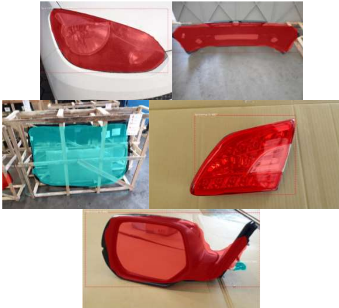
Figure 6. Image segmentation for the automotive parts proposed in this work
